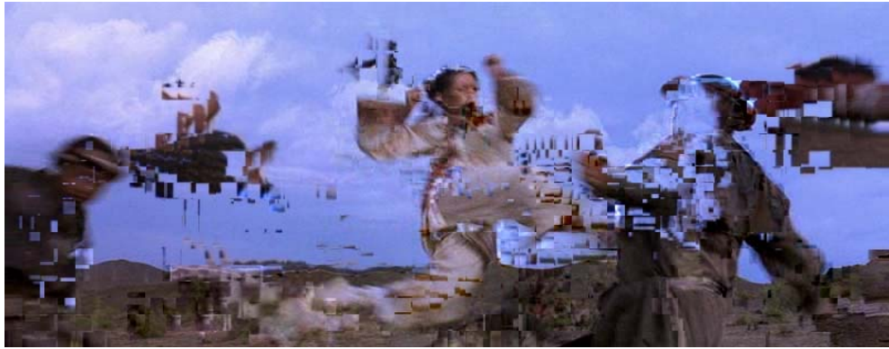
Figure 5: Mpeg4, Drop = 0.1%, Delay = 1.5 ms and Jitter = 0.025 ms
