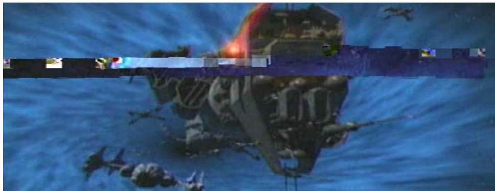
Figure 6: Mpeg2, Drop = 0.1%, Delay = 1.5 ms and Jitter = 0.025 ms
